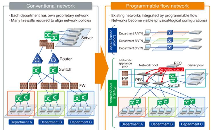
VTN: Virtual tenant network FW: Firewall PFC: Programmable flow controller PFS: Programmable flow switch
