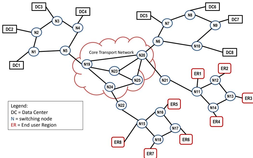
**Figure A.1 – Example transport network physical topology**
