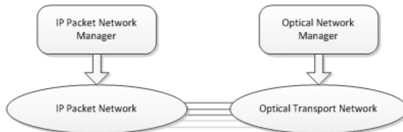
**Figure 8 – Independent operation of packet and optical networks**
