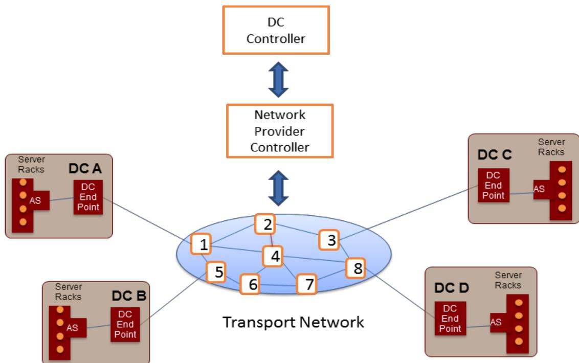
**Figure 6 – Data center interconnection architecture**
