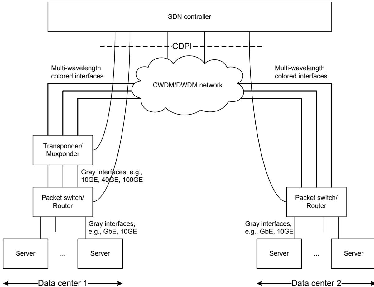
**Figure 1 – Data center interconnect, all-optical network**
