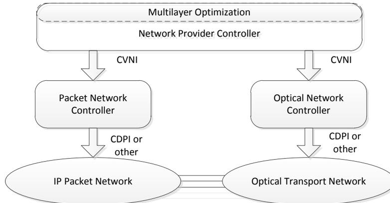
**Figure 11 – Multi-layer control with separate packet services and optical network controllers**
